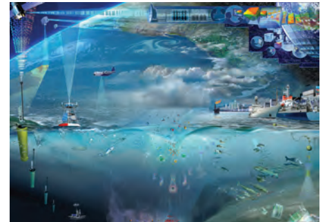
An illustration of the components of the Global Ocean Observing System. The national system is modeled on a similar framework.
